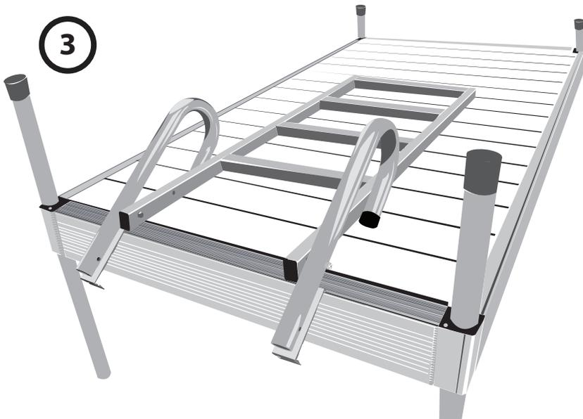
Lay the assembled ladder on the dock in the flipped up position so you do not have to hold it while trying to attach it. Having it assembled will space the handles the right distance apart from each other.
