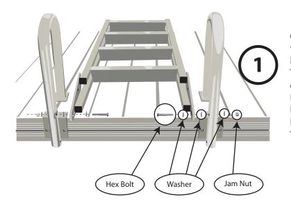
Connect the ladder hoops to the oblong holes with the ladder between each ladder hoop. Use two hex bolts and two nylock jam nuts from the bolt kit bag. Threaded ends of all bolts should point to the outside of the ladder to avoid the path of swimmers. Place a stainless washer on the ends of the bolts and between the ladder and the hoop to allow the Ladder to swing up and down without grinding. Tighten nuts and bolts before using the ladder.
