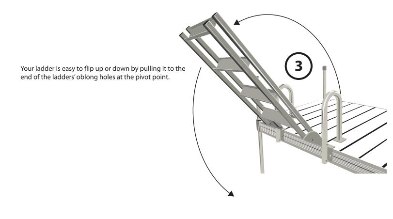
Retract the "Ladder Spring Pins" to get the ladder in the down position. You can offset the pin in the hole to hold the spring while swinging the ladder down. Release the pin from the offset position to keep the ladder from moving while in the down position.
