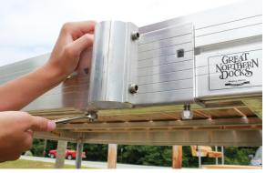
2. Apply two nylock nuts attaching the pipe bracket to the Frame of the dock.
