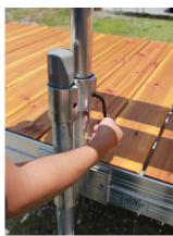
6. Set the bench legs down into the double sockets and tighten all set screws.
