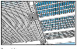
Step 10 Once the legs are installed, secure the section to the J brackets by tightening the 3/8" nuts.
