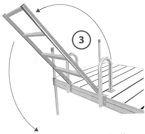
Once the ladder is bolted to the handles and the handles are bolted to the dock, you should be able to swing the ladder up and over. Keep hands free and clear from being pinched while the ladder is in motion. To prevent motion and pinching, there is a spring pin located in the lower part of the ladder handle.
