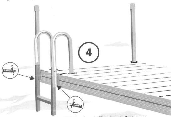
To make it easy to get the spring pins into the ladder, pull them back and offset them in the hole so they will not spring back. You can then swing the ladder to the down position and release the spring pins through the holes in the handles and into the holes on the ladder.
