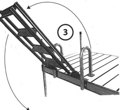
Your ladder is easy to flip up or down by pulling it to the end of the ladders' oblong holes at the pivot point.
