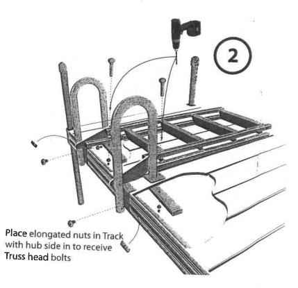
Lay the assembled ladder on the deck the flipped up position so you do not have to hold it while trying to attach it.
