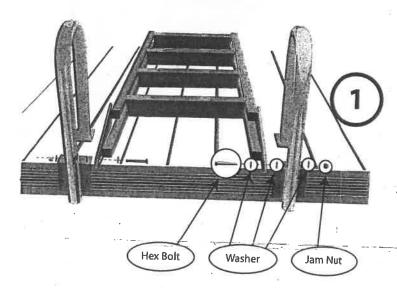
Connect the ladder hoops to the oblong holes with the ladder between each ladder hoop. Use two hex bolts and two nylock jam nuts from the bolt kit bag. Threaded ends of all bolts should point to the outside of the ladder to avoid the path of swimmers. Place a stainless washer on the ends of the bolts and between the ladder and the hoop to allow the Ladder to swing up and down without grinding. Tighten nuts and bolts before using the ladder.
